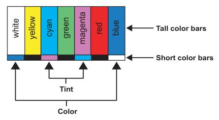
**TINT** (also known as 'hue') is essentially the ratio of red to green in the color portion of the image. If TINT is decreased, the image will appear redder, and increasing it will cause the image to appear greener. To set TINT properly, look at the color bar pattern through a blue filter (or mute the red and green outputs). Adjust TINT until the middle two tall color bars match the middle short color bars (see color bar drawing).
